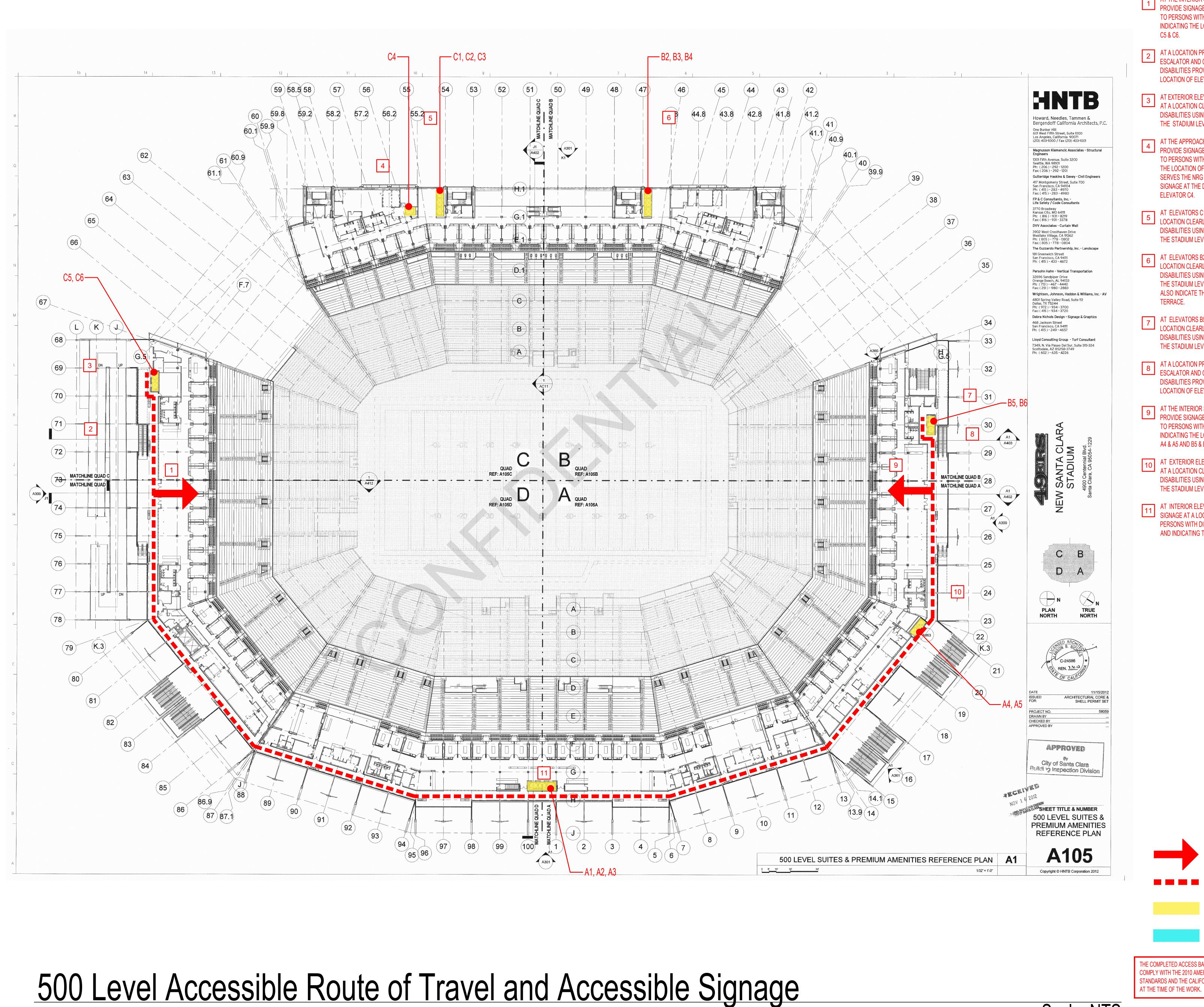
AT THE INTERIOR SIDE OF LOBBY ENTRY/EXIT DOORS PROVIDE SIGNAGE AT A LOCATION CLEARLY VISIBLE TO PERSONS WITH DISABILITIES USING A WHEELCHAIR INDICATING THE LOCATION OF EXTERIOR ELEVATORS C5 & C6.
