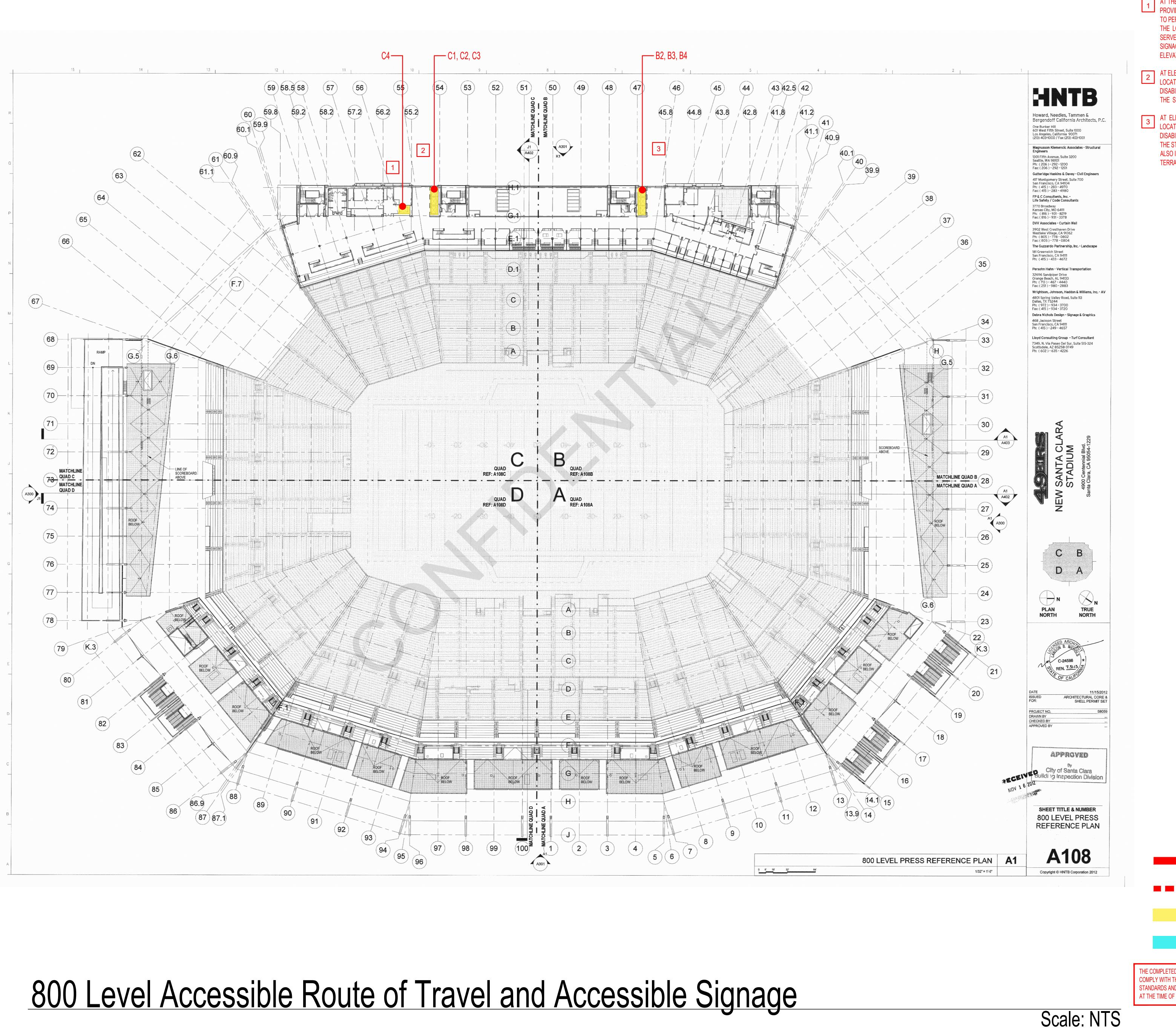
AT THE APPROACH TO ELEVATORS C1, C2, & C3 PROVIDE SIGNAGE AT A LOCATION CLEARLY VISIBLE THE LOCATION OF ELEVATOR C4 AND INDICATE IT SERVES THE NRG TERRACE. ALSO PROVIDE SIMILAR SIGNAGE AT THE DOOR LEADING TO THE LOBBY OF ELEVATOR C4.
