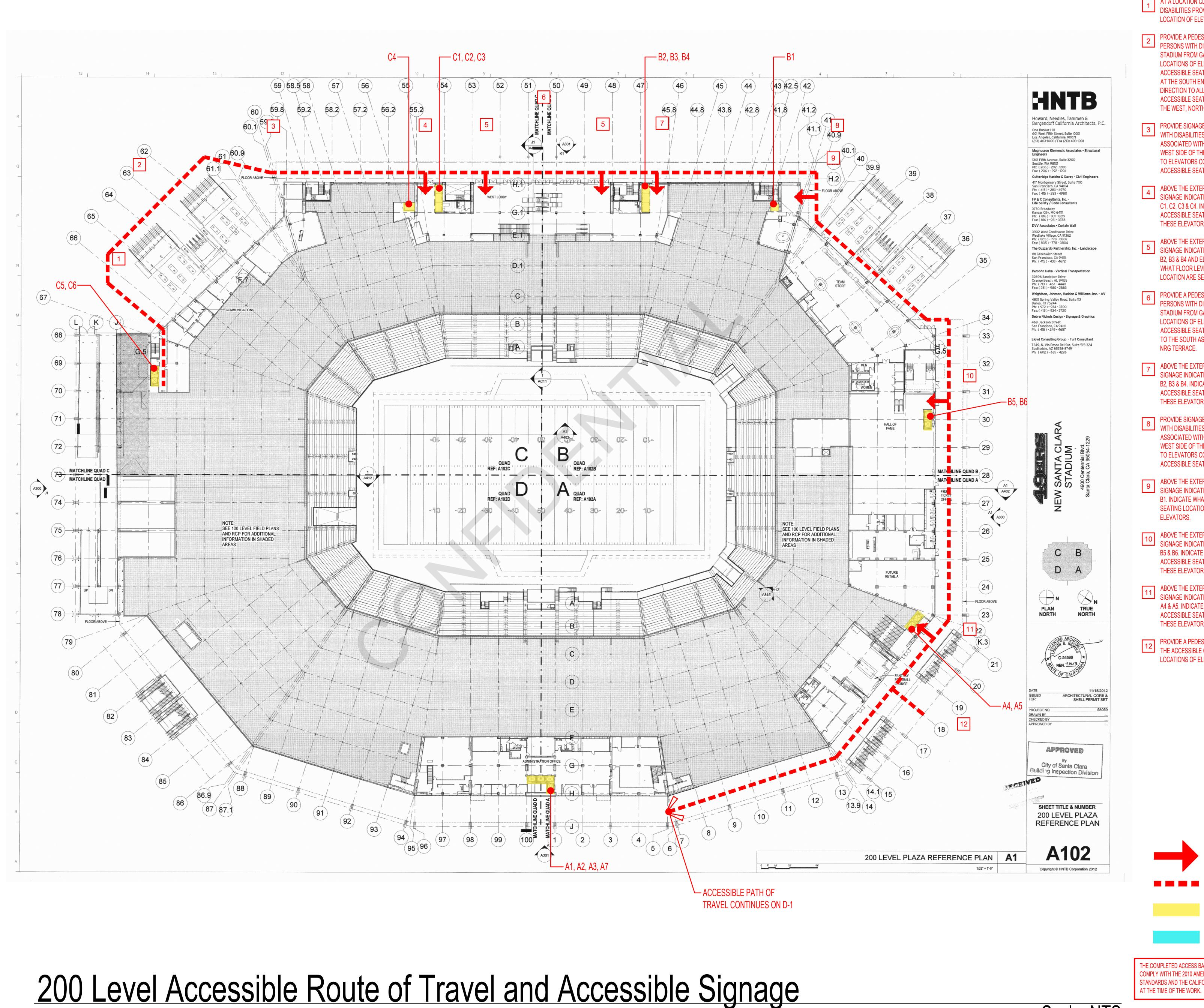
AT A LOCATION CLEARLY VISIBLE TO PERSONS WITH DISABILITIES PROVIDE SIGNAGE INDICATING THE LOCATION OF ELEVATORS C5 & C6.
