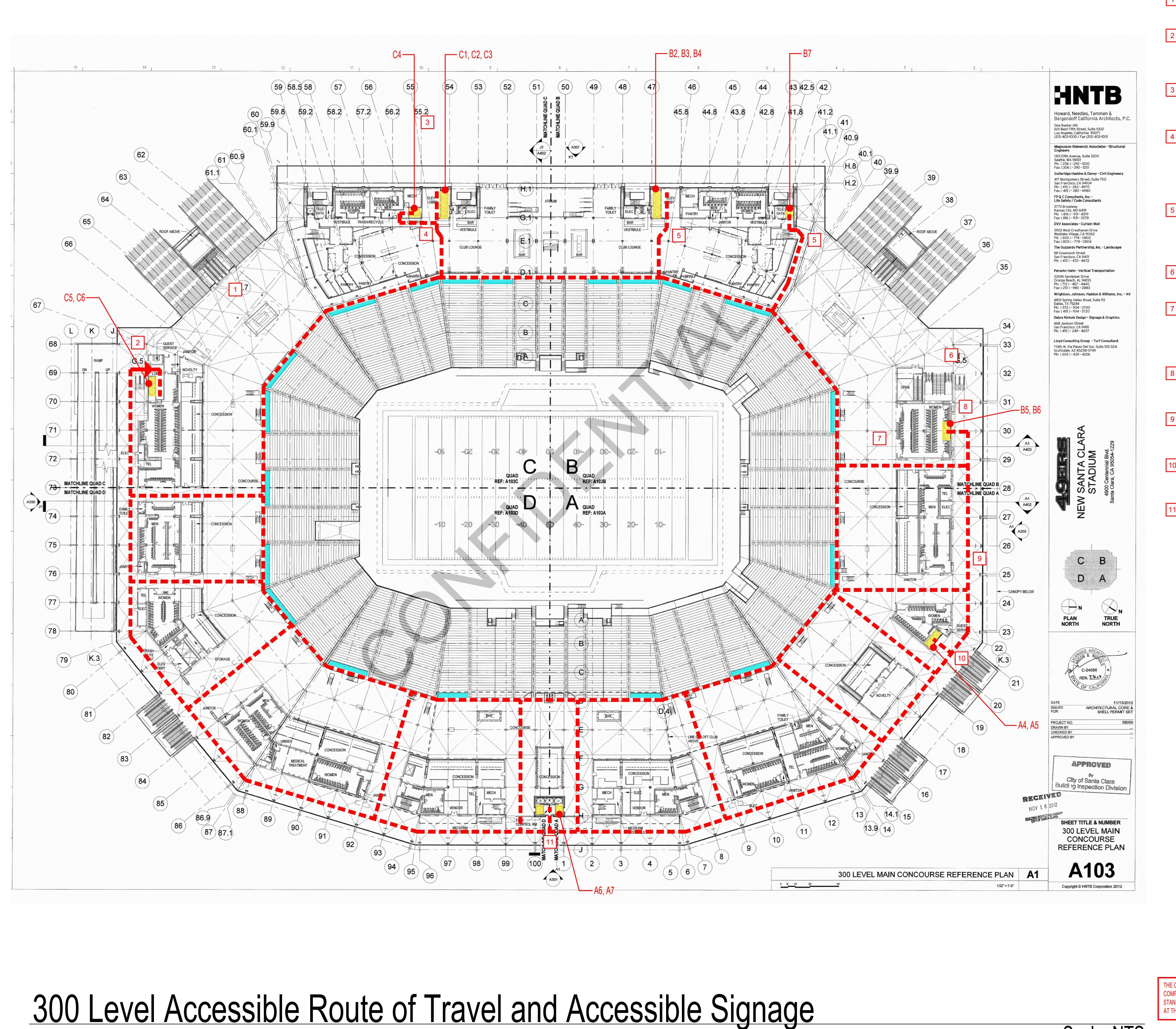
AT THE ESCALATORS PROVIDE A SIGN CLEARLY VISIBLE TO PERSONS WITH DISABILITIES USING A WHEELCHAIR THE LOCATION OF ELEVATORS C5 & C6.
